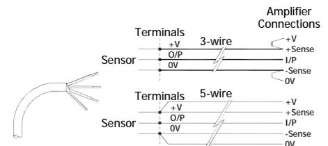
Sensors supplied with cable are calibrated with the cable fitted which negates errors due to conductor resistance at room temperature; however, small gain errors due to temperature fluctuations in the cable should be expected.
